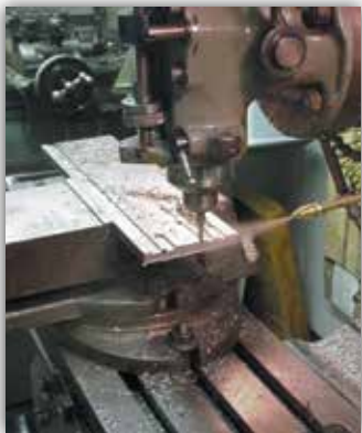
Spray cooling during milling operation
