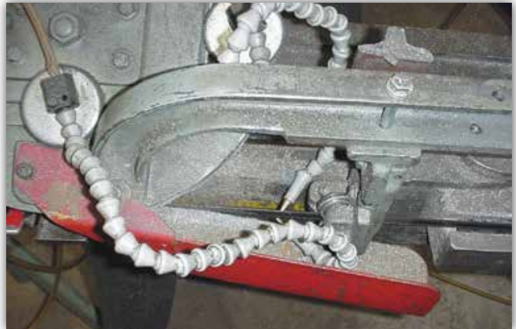
Minimum quantity lubrication used on a horizontal saw
