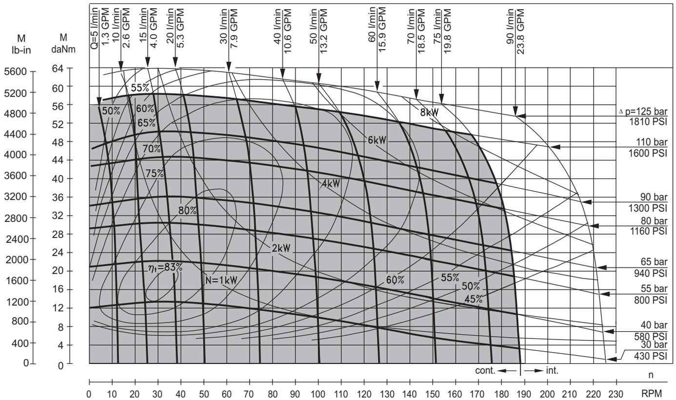
The function diagrams data is for average performance of randomly selected motors at back pressure  $5 \pm 10$  bar [72.5  $\pm$  145 PSI] and oil with viscosity of 32 mm<sup>2</sup>/s [150 SUS] at 50°C [122°F].
