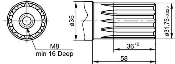
**CB** -  $\varnothing 35$  straight, Parallel key A10x8x45 DIN 6885
