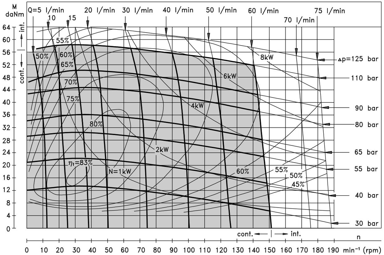
The function diagram data was collected at back pressure 5 ÷ 10 bar and oil with viscosity of 32 mm<sup>2</sup>/s at 50° C.
