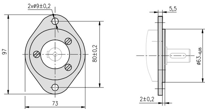
Flange Kit includes 3 screws - M6x14 for attaching flange to the motor.
