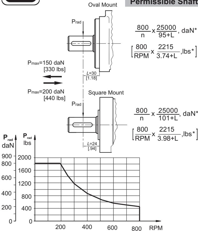
Radial Shaft Load  $P_{\text{rad}}$  for C, CO Shaft Extensions by  $L=30 \text{ mm}$  [1.18 in] (24 mm [.94 in])
