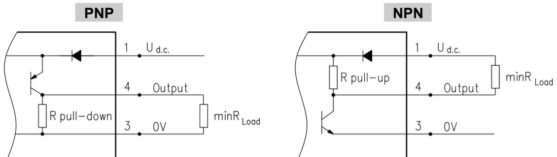
$$R_{Load} = U_{d.c.} / I_{max} (=50\text{mA})$$
