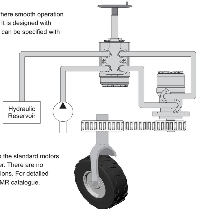
The main technical features correspond to the standard motors series MR  $\varnothing 28,56$  [1.124 in.] sealing diameter. There are no changes in the overall and mounting dimensions. For detailed technical and mounting data please refer to MR catalogue.
