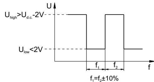
Load max.:  $I_{high} = I_{low} < 50\text{mA}$
