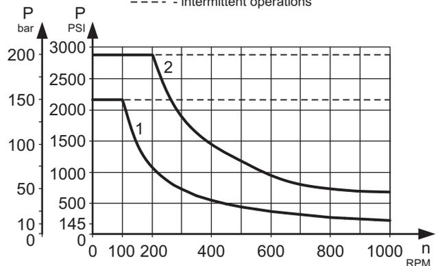
1: Curve for Standard Shaft Seal
