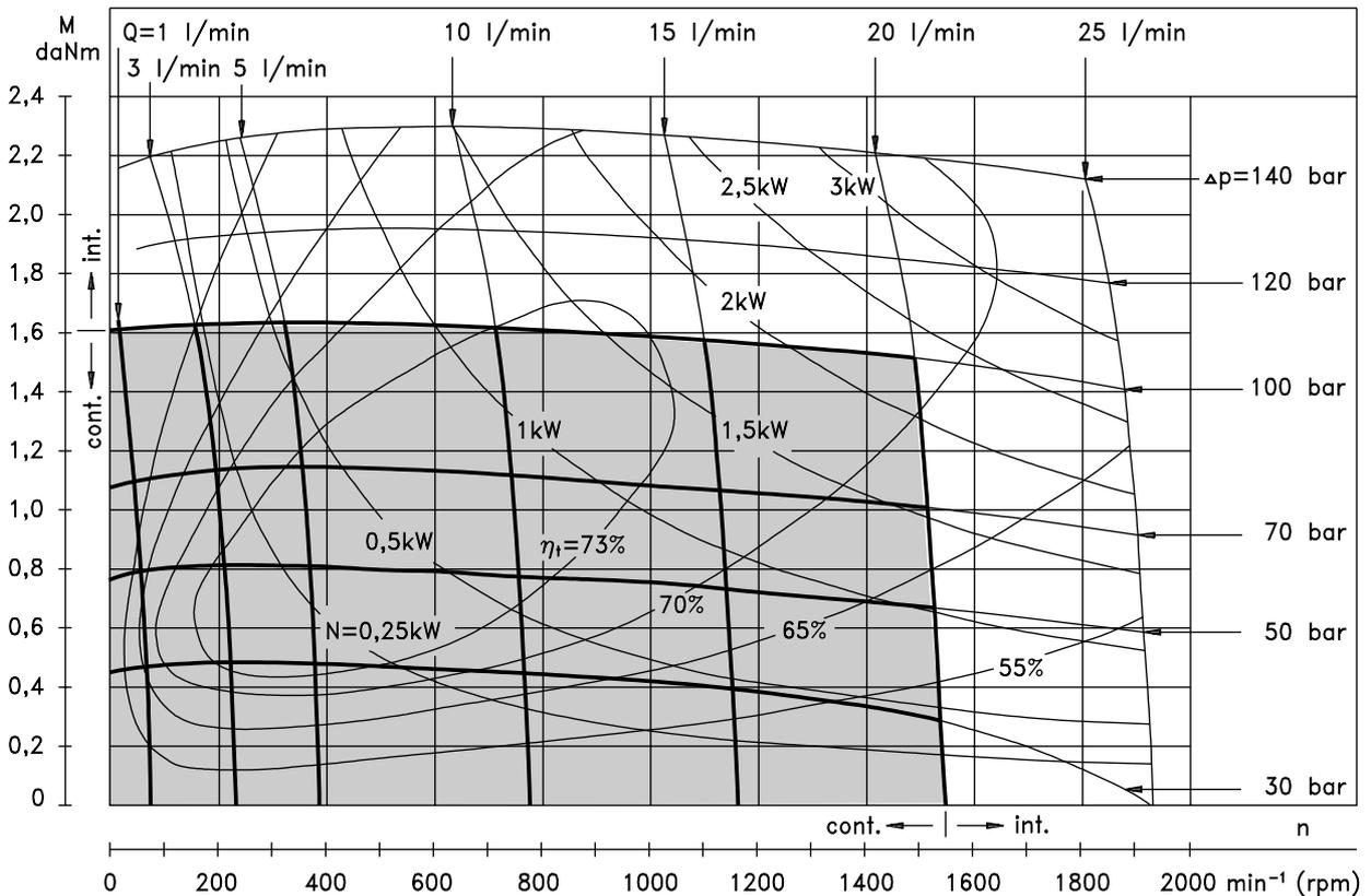
The function diagrams data was collected at back pressure 5÷10 bar and oil with viscosity of 32  $\text{mm}^2/\text{s}$  at 50° C.
