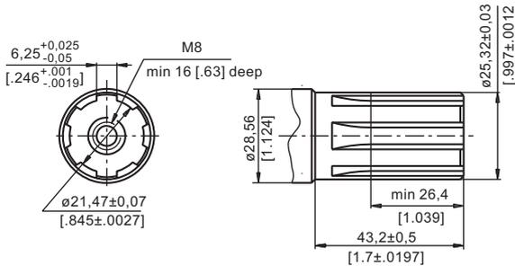
**K** - tapered 1:10, Parallel key B5x5x14 DIN 6885
