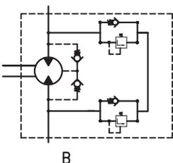
**HW... motors with drain connection:**
