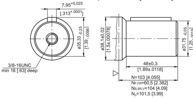
**M** - 32 straight, Parallel key A10x8x32 DIN 6885
