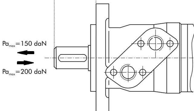
Radial Shaft Load  $P_{rad}$  for C, CO Shaft Extensions by  $L = 30 \text{ (24) mm}$
