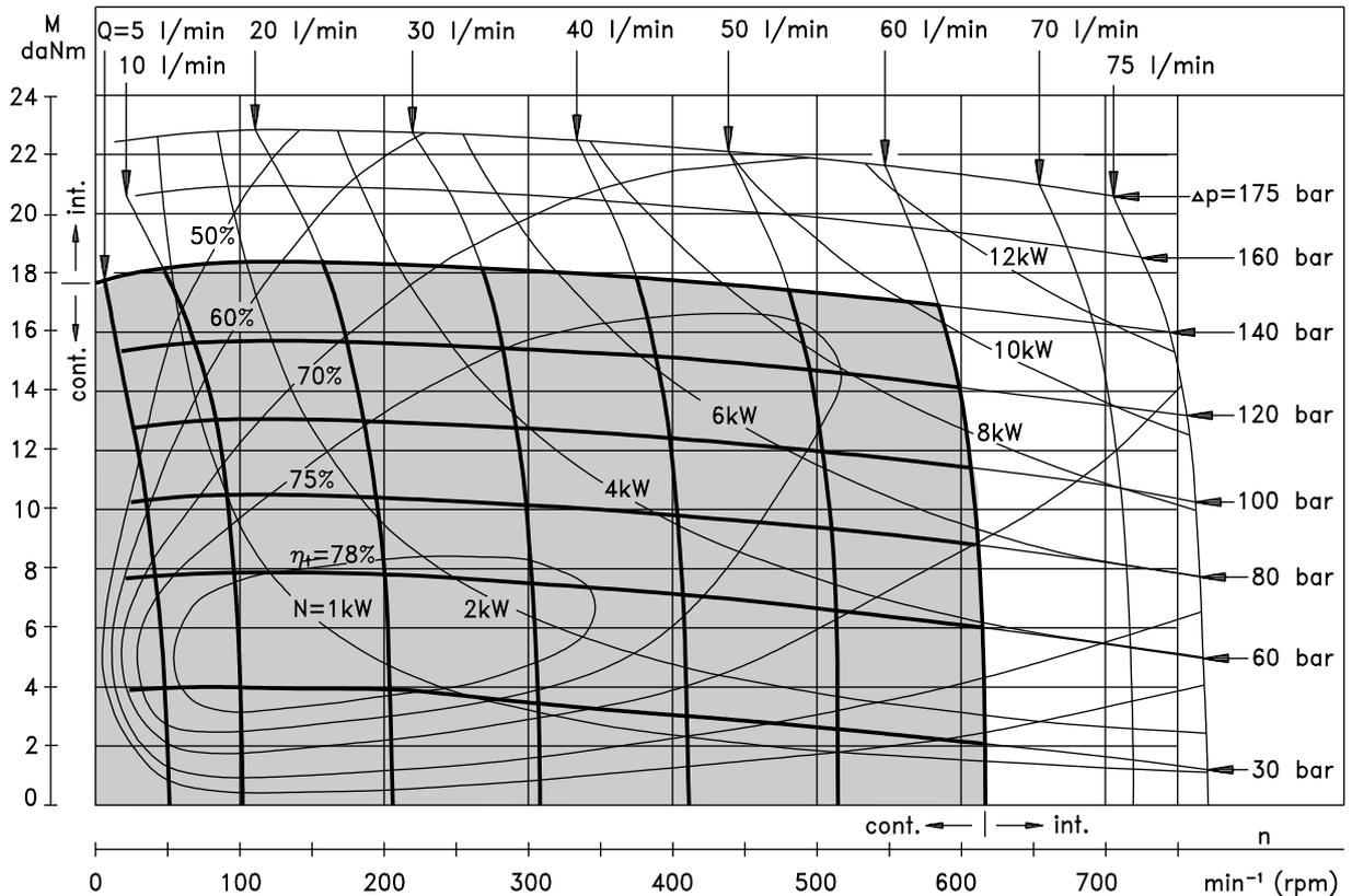
The function diagrams data was collected at back pressure 5 ÷ 10 bar and oil with viscosity of 32 mm<sup>2</sup>/s at 50° C.
