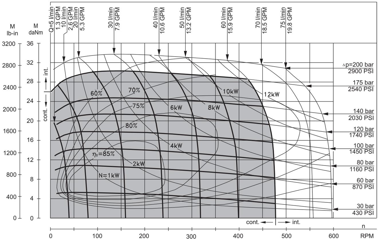
The function diagrams data is for average performance of randomly selected motors at back pressure  $5 \pm 10$  bar [72.5  $\pm$  145 PSI] and oil with viscosity of  $32 \text{ mm}^2/\text{s}$  [150 SUS] at  $50^\circ\text{C}$  [122 $^\circ\text{F}$ ].
