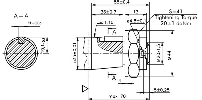
**K** - tapered 1:10, Parallel key B5x5x14 DIN 6885
