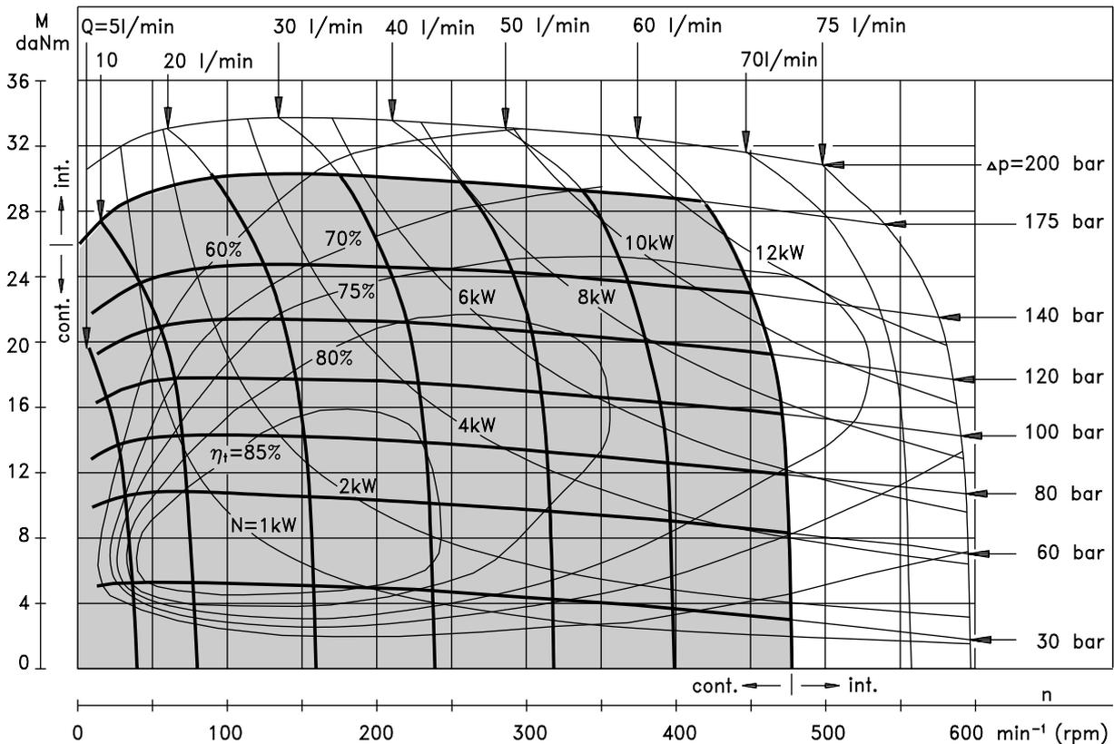
The function diagrams data was collected at back pressure  $5 \div 10 \text{ bar}$  and oil with viscosity of  $32 \text{ mm}^2/\text{s}$  at  $50^\circ \text{ C}$ .
