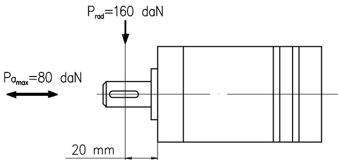
The permissible radial shaft load [P<sub>rad</sub>] is calculated from the distance [L] between the point of load application and the mounting surface:
