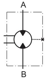
MRNA is suitable for driven mechanism where smooth operation low speed and high pressure is demanded. It is designed with separated output shaft and spool valve and can be specified with low internal leakage.
