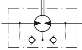
**RW...U motors with high pressure seal and drain connection:**
