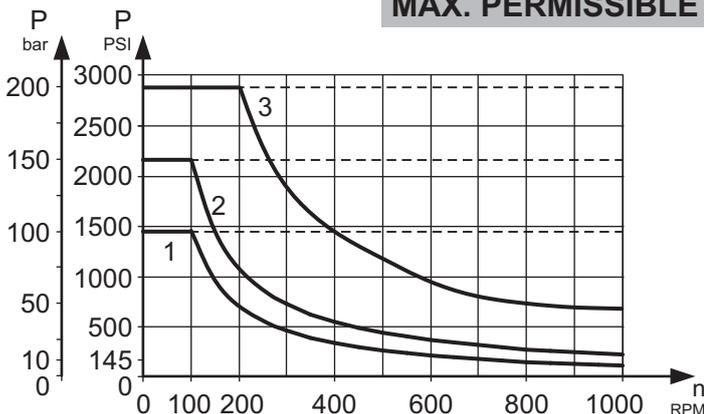
Max return pressure without drain line or max. pressure in drain line
