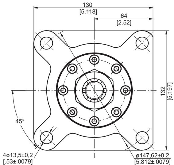
P<sub>(A,B)</sub>: 2xG1/2 or 2xM22x1,5 - 17 mm [.67 in.] depth
