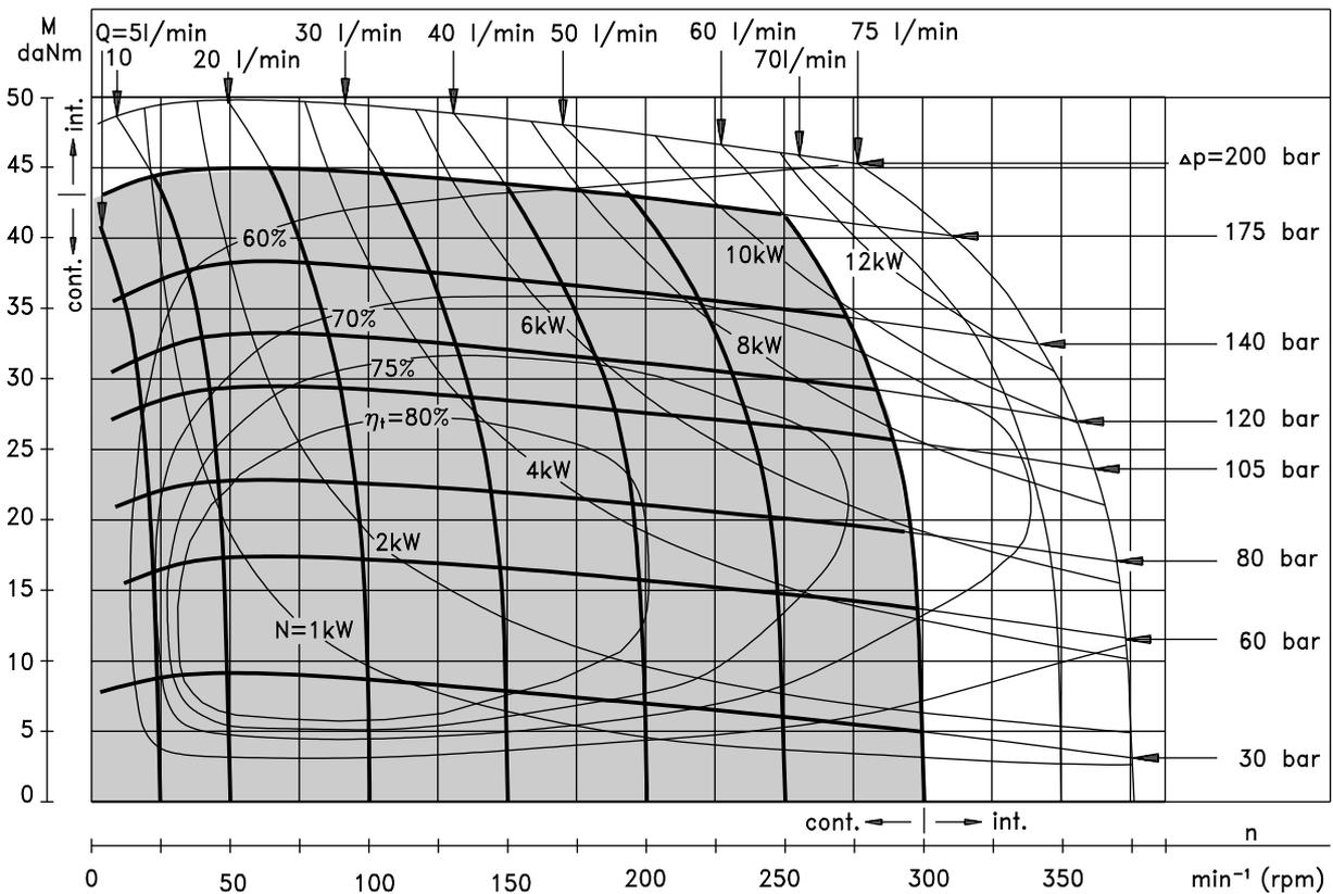
The function diagrams data was collected at back pressure  $5 \div 10$  bar and oil with viscosity of  $32 \text{ mm}^2/\text{s}$  at  $50^\circ \text{C}$ .
