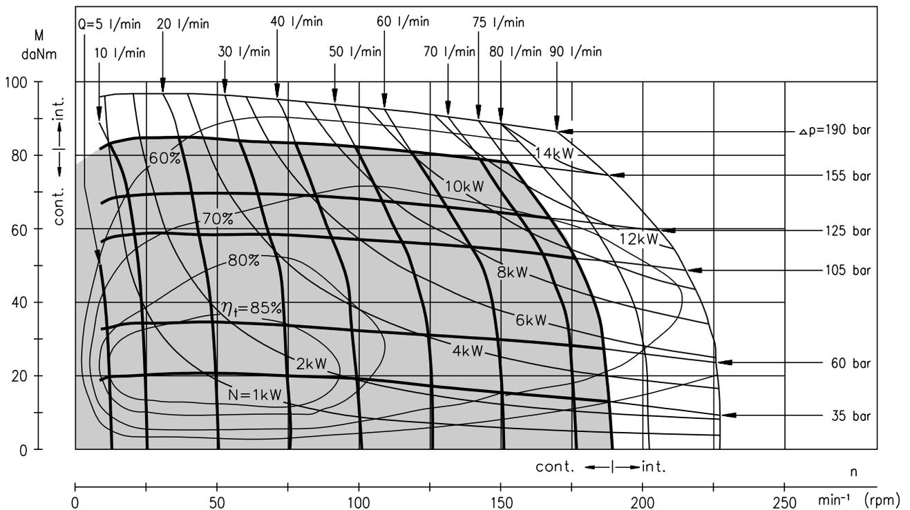
The function diagrams data was collected at back pressure 5 ÷ 10 bar and oil with viscosity of 32 mm<sup>2</sup>/s at 50° C.
