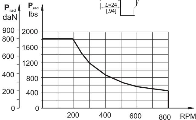
Radial Shaft Load  $P_{rad}$  for C, CO Shaft Extensions by  $L=30 \text{ mm}$  [1.18 in] (24 mm [0.94 in])
