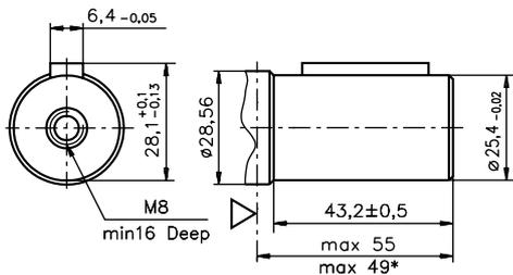
**SB** - splined A25x22xH10 DIN 5482
