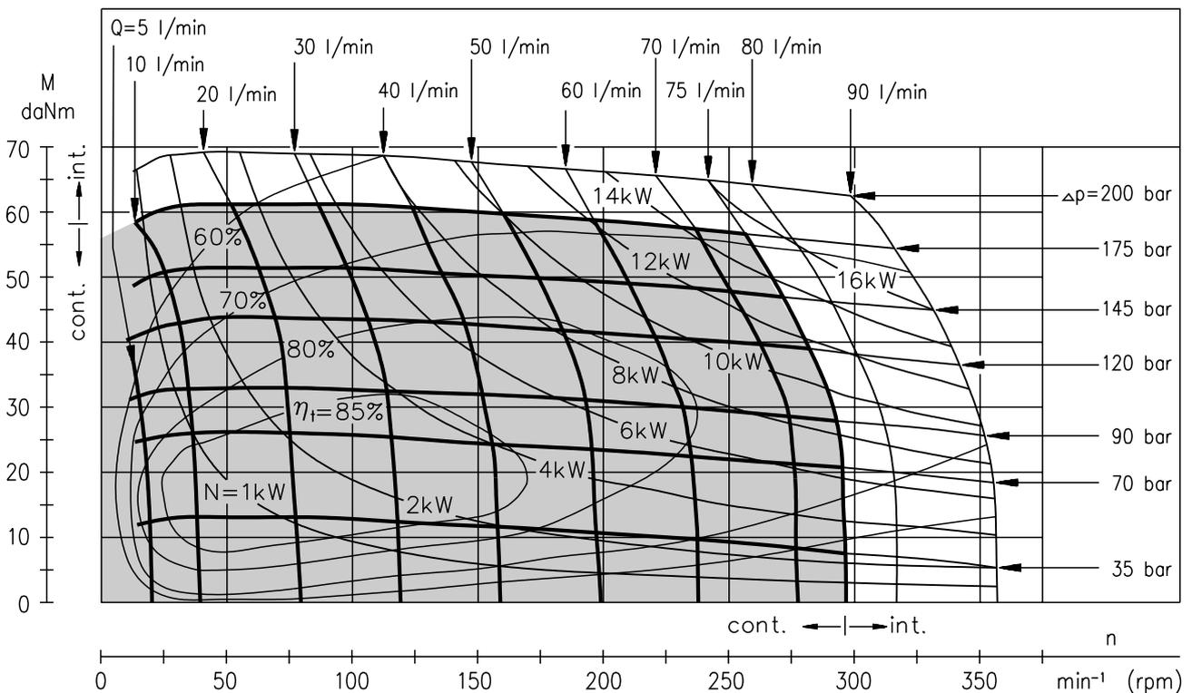
The function diagrams data was collected at back pressure 5 ÷ 10 bar and oil with viscosity of 32 mm<sup>2</sup>/s at 50° C.
