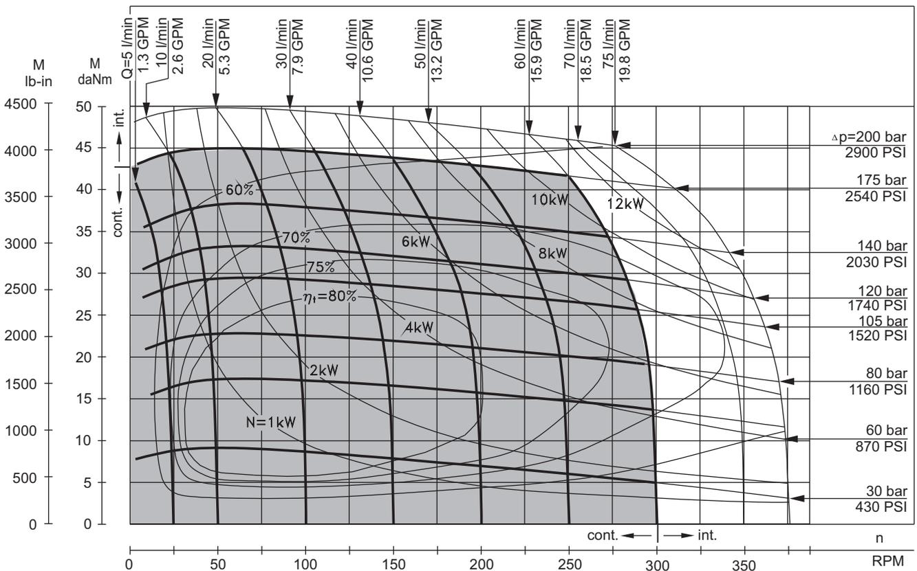
The function diagrams data is for average performance of randomly selected motors at back pressure  $5 \pm 10$  bar [72.5  $\pm$  145 PSI] and oil with viscosity of 32 mm<sup>2</sup>/s [150 SUS] at 50°C [122°F].
